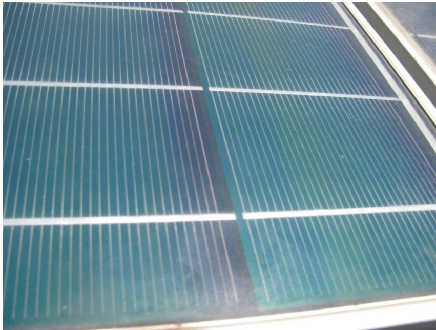
Fig. 8.34: Light yellow discoloration seen in CIGS module
