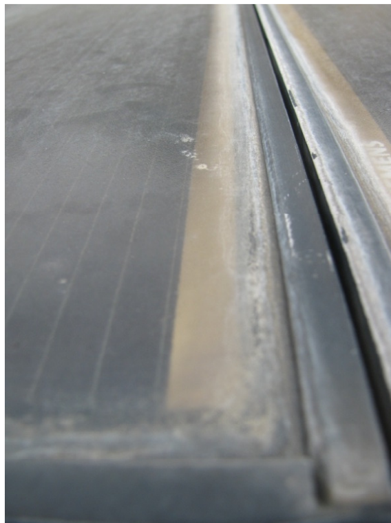
Fig. 8.36: Dark patches close to electrode of CIGS module
