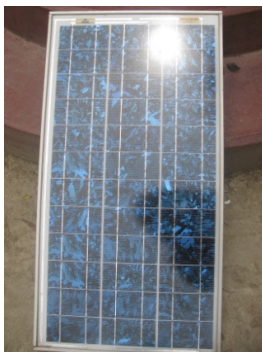
No Discoloration or delamination
