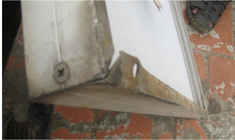
Fig. 8.31: Corroded and dented frame of a PV module
