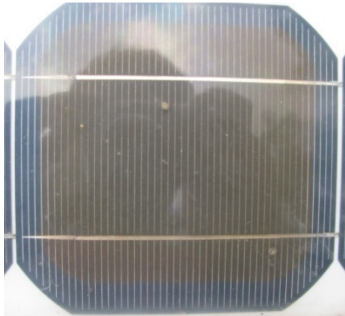
Fig. 8.7: Browning of EVA from the centre with transparent EVA intact at the edge of the solar cell
