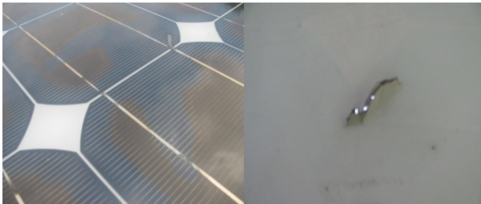
Fig. 8.8: Uneven discoloration (left) in a module and puncture in the back-sheet (right) of same module.
