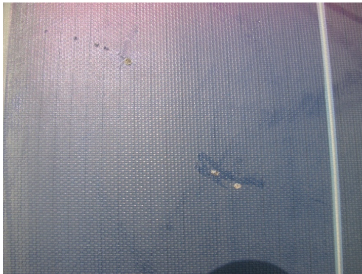
Fig. 8.45: Puncture marks on the module top fabric
