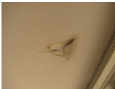
Scratches in backsheet
