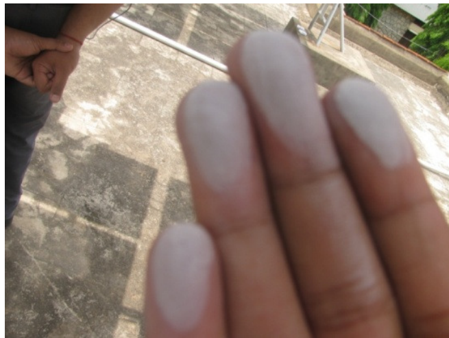
Fig. 8.24: White powder from backsheet of a module
