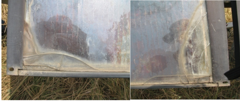
Fig. 8.40: Cracks in the glass of the corroded module
