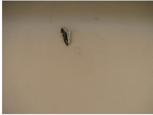
Fig. 8.37: Puncture in the backsheet of the CIGS module
